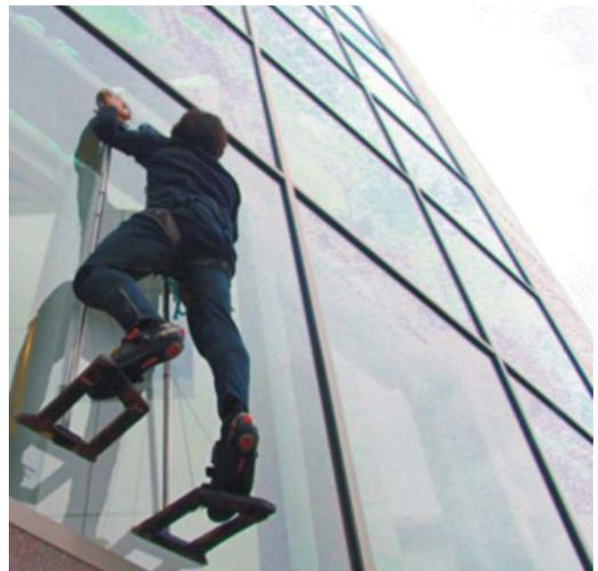
Researchers at Stanford University led by engineer Mark Cutkosky have come up with a gecko-inspired human climbing system that they hope to use in manufacturing equipment, making grippers for manipulating huge solar panels, displays, and other objects without the need for suction power or chemical glues. The team is also working with NASA's Jet Propulsion Laboratory to adapt the adhesive for use by robots.
