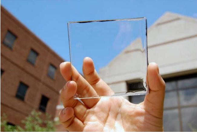
Researchers at the Michigan State University has developed a new type of solar concentrator that when placed over a window creates solar energy while allowing people to actually see through the window. It is called a transparent luminescent solar concentrator and can be used on buildings, cell phones and any other device that has a clear surface.
