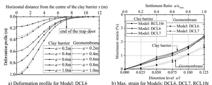
Figure 2. Deformation profiles and strain variation for clay barrier and geomembrane at different settlement stages.
