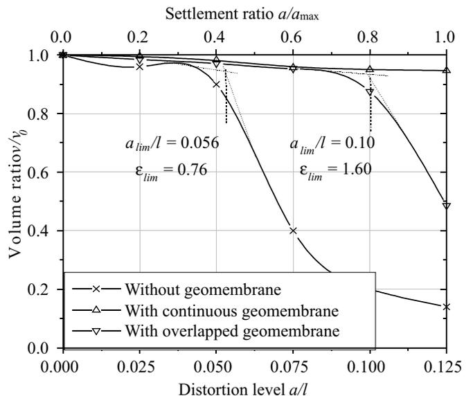
Figure 3. Variation of volume ratio with distortion level  $a/l$  and settlement ratio  $a/a_{max}$ .
