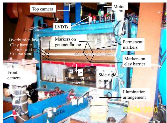
Figure 1. Centrifuge model test setup
