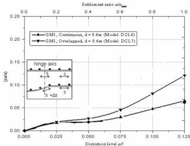
Figure 4. Variation of  $(s/s)$  with  $a/l$  and  $a/a_{max}$  for barriers with continuous and overlapped geomembrane
